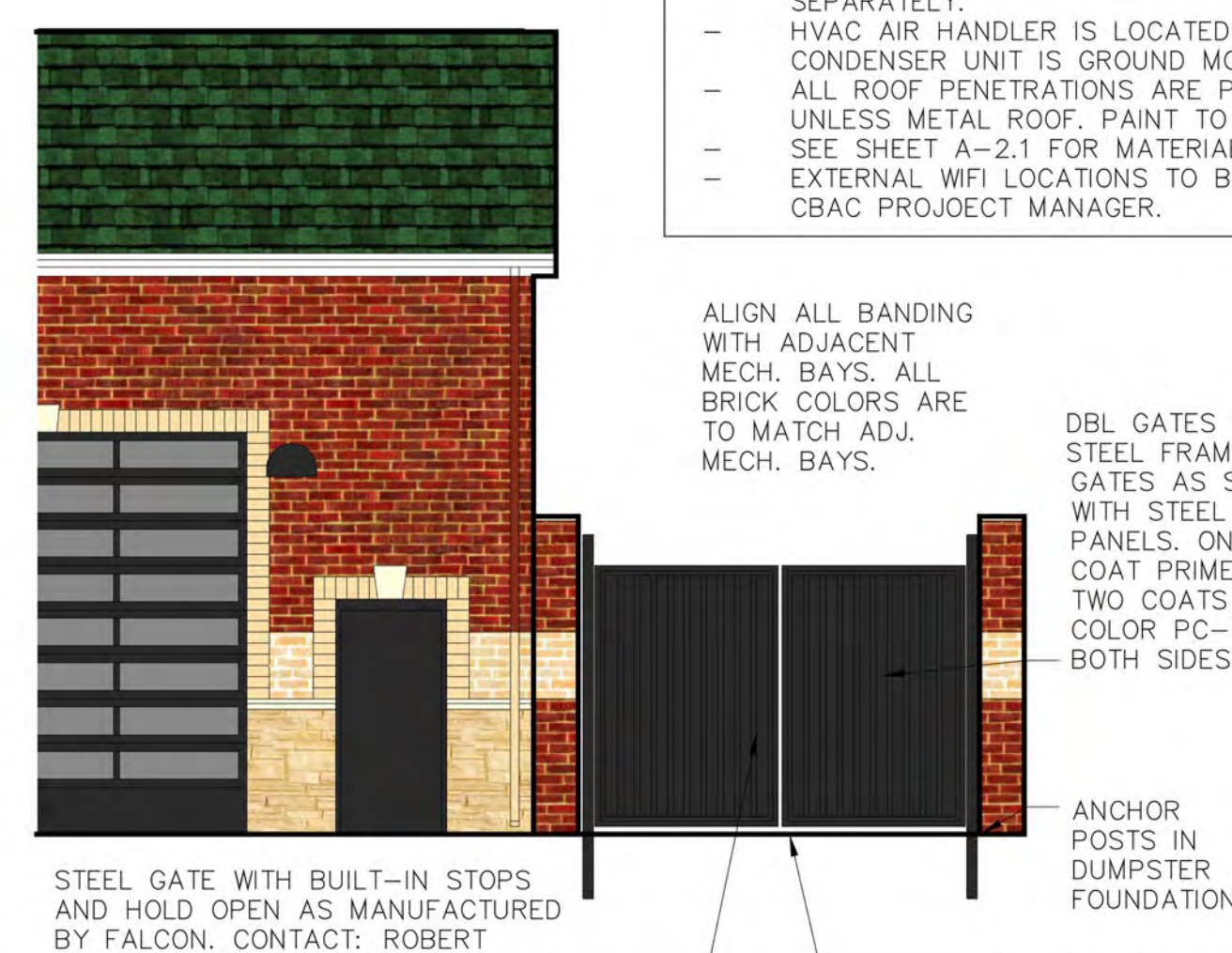
1 DUMPSTER ENCLOSURE ELEVATION SCALE: 3/16" = 1'- 0"
