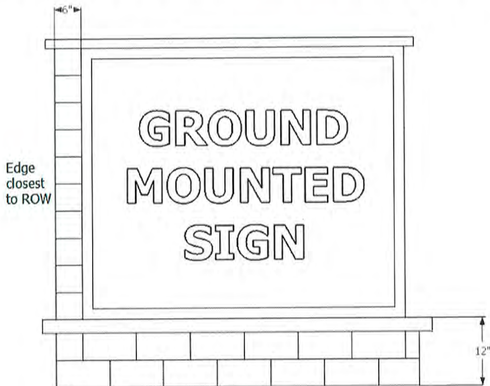
Figure 165.18-3 Ground-Mounted Signs Perpendicular to the Right-of-Way
