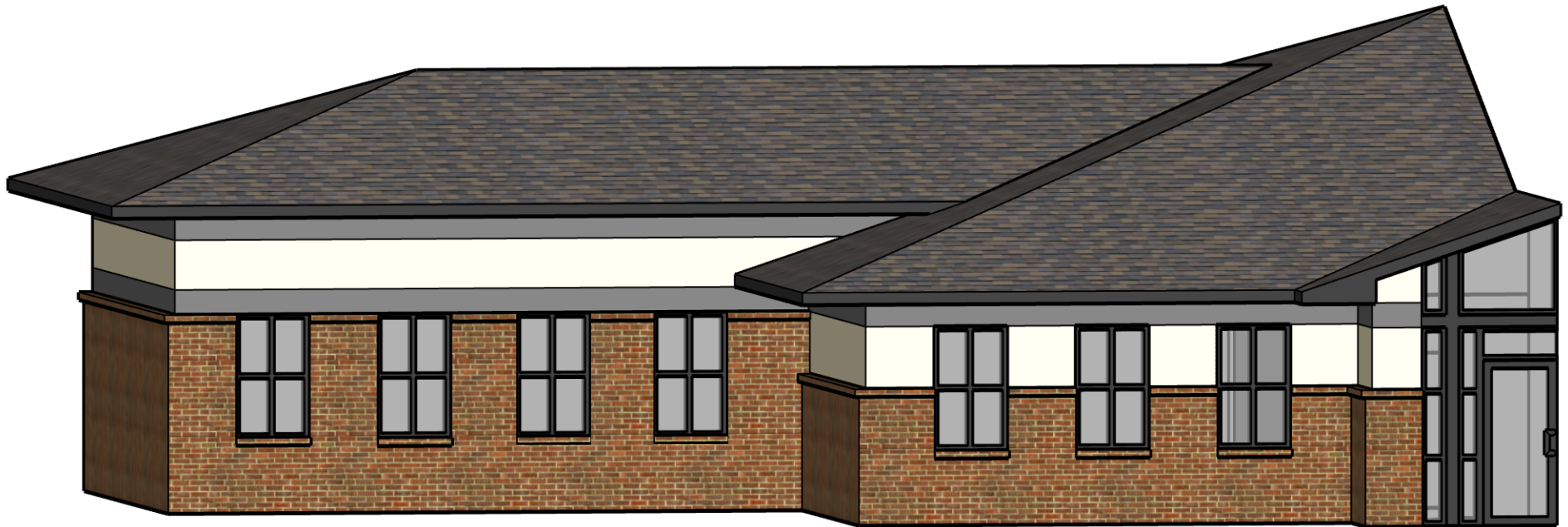
75% Brick Matching Current Brick, South Elevation
