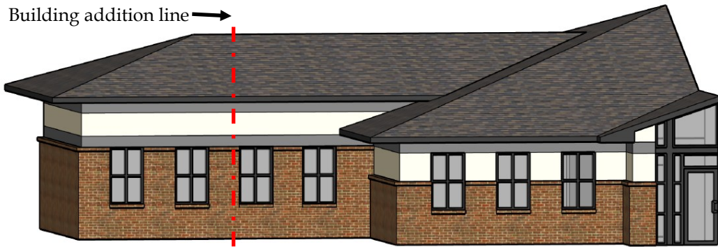
75% Brick Matching Current Brick, South Elevation
