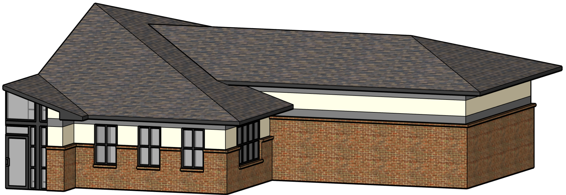
75% Brick Matching Current Brick, North Elevation
