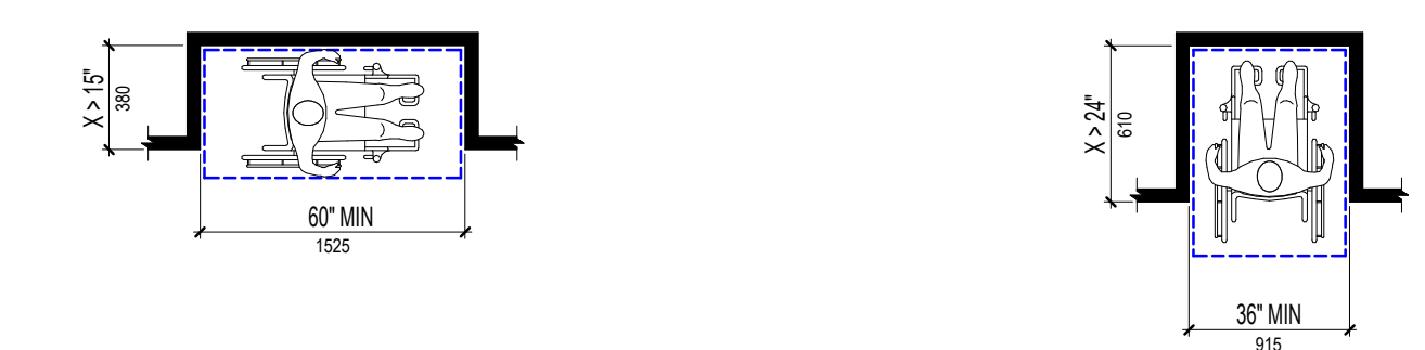
8 Maneuvering Clearance in an Alcove, Parallel Approach A.0-2 1/4" = 1'-0" 9 Maneuvering Clearance in an Alcove, Forward Approach A.0-2 1/4" = 1'-0"
